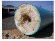
When FOG is washed down the drain, it doesn't vanish. It travels through the sewer pipes and laterals, trapping food particles and other debris, and GROWS!! This can cause clogs in pipes, overflows, and backups in homes and public sewers, harming the environment.
